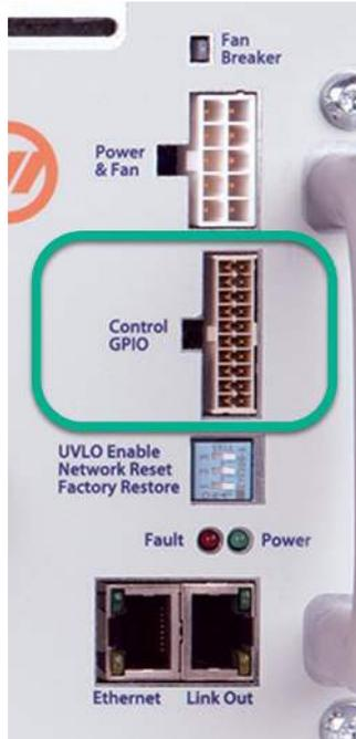
**Figure 34. Control GPIO port**
