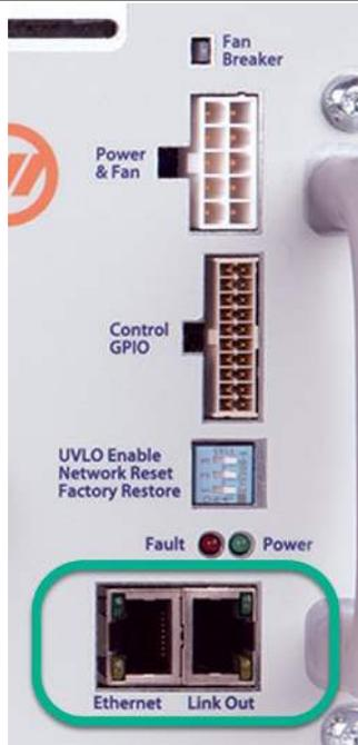
**Figure 38. Link Out Connector**
