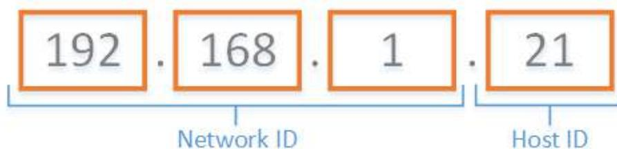
**Figure 42. Parts of an IP address**
